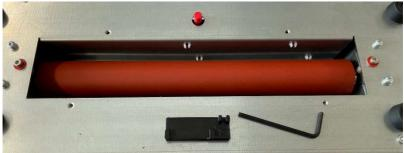
5.) After cleaning, the unit should first be well ventilated with the cleaning cover open and only put back into operation when no more moisture from the cleaning agent can be detected. Then close the cover.
